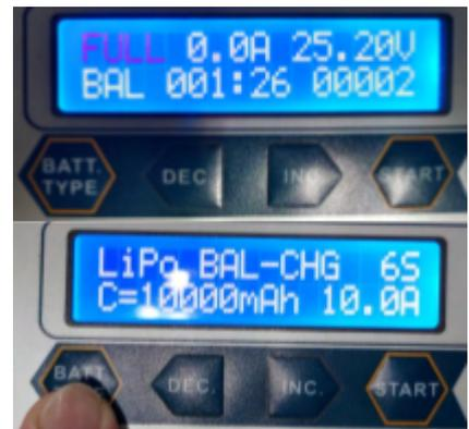
To check the voltage value on each individual cell, press "INC" while the battery is charging.
