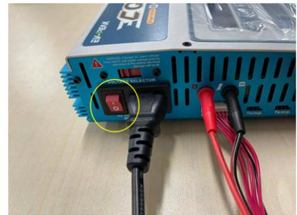
Using the XT90 and balance port connectors, connect the batteries to be charged to the charger.
